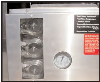
New dispenser and heater housing (provides easy access from the front and additional protection).
