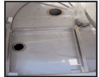
New strategic locations for wash and rinse tank drains (clear rinse flow with separation of wash and rinse tanks).
